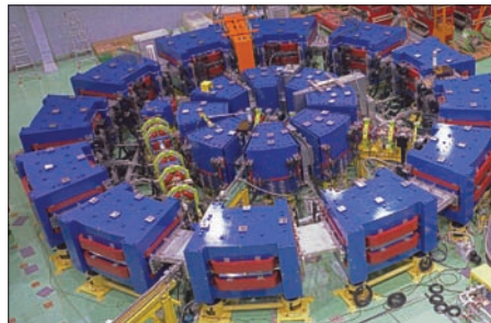
The proton FFAG accelerator. (Courtesy KURRI.)
